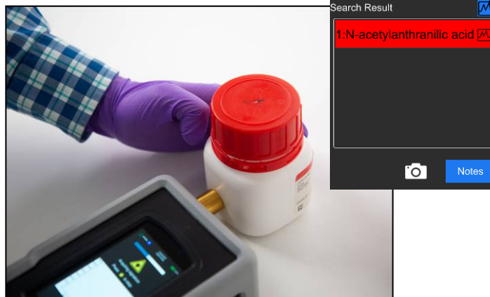
Fig. 4 TacticID-1064 ST measurement through HDPE bottle and match result for N-acetylanthranilic acid
