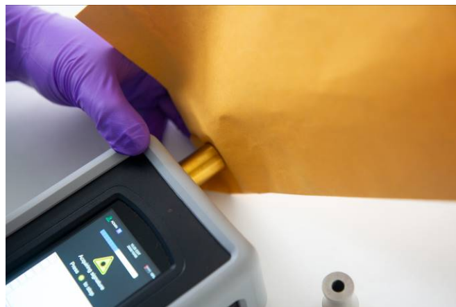
Fig. 1 TacticID-1064 ST measuring a sample through a manila envelope with ST adapter
