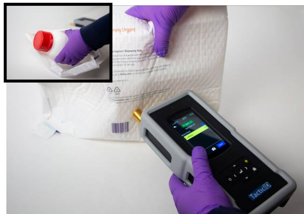
Fig. 5 Measurement of white HDPE bottle of caffeine inside white padded package
