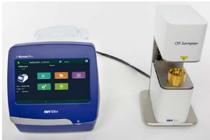
Fig 2. QTRam portable Raman spectrometer with the QT-Sampler for transmission Raman measurements. BWAnalyst software (shown on the QT Ram) was used for all analyses.
