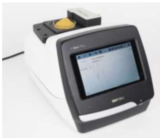
Fig. 1 i-Spec ® Plus Diffuse Reflectance Portable NIR Spectrometer with turntable
