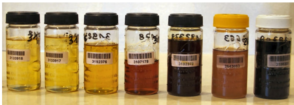
Figure 3: An illustrative series of samples showing aging, oxidation and dispersed water
