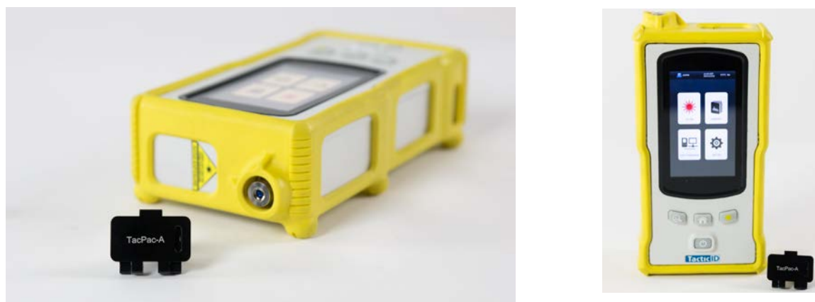
Fig. 2 TacticID handheld Raman spectrometer with 785-nm laser excitation and TacPac adaptor
